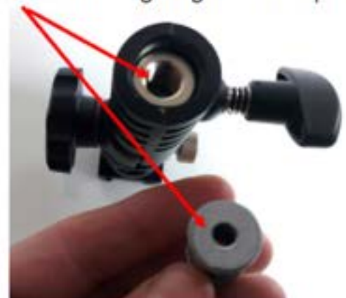
Screw thread for lighting stand or tripod
